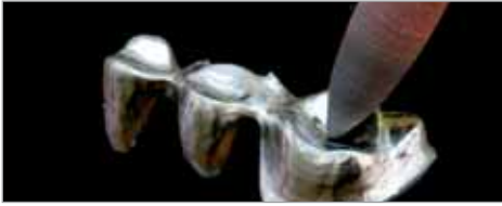
Fig. 40 Before sandblasting using 110 micron aluminum oxide, the entire frame work surface is smoothed, using a silicone polisher to avoid any sharp edges and also to detect any casting porosities and to eliminate any metal folds (especially when soft, high-gold bio-alloys are used), which could result in bubbles or cracks in the porcelain.
