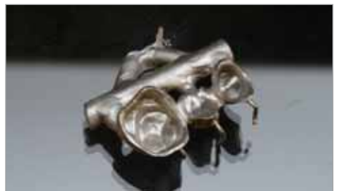
Fig. 28 Devested casting using a standard palladium containing precious bonding alloy. Note the fine surface that GC Fujivest Platinum yields.
