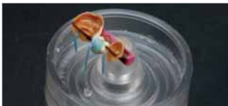
Fig. 27 A ringless casting system can be used with GC Fujivest Platinum for equal and unhindered expansion of the investment and to keep metal oxide contamination of the burnout furnace at a minimum if it is also used for burning out rings for pressable ceramics.
